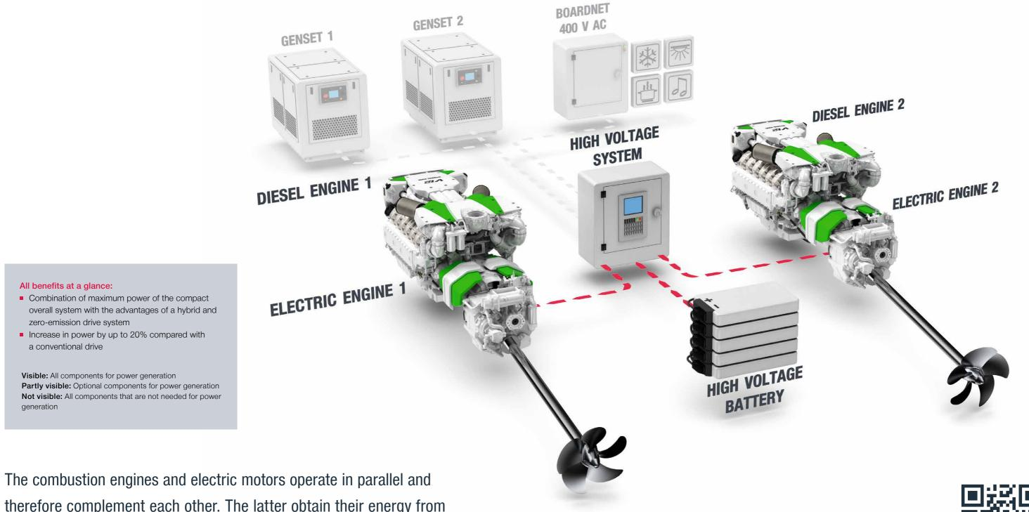
therefore complement each other. The latter obtain their energy from the batteries. The interaction of both energy sources means that the absolute maximum power output can be achieved in this operating mode.
